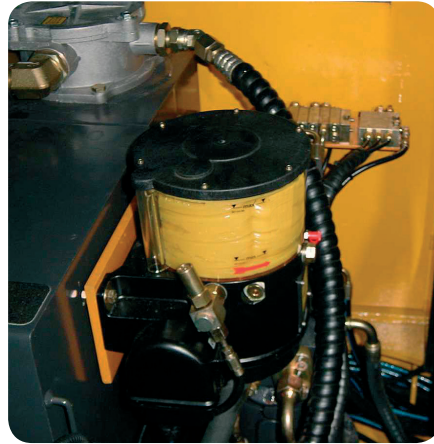
Pump unit with integral control electronics on a KOMATSU PC110.
