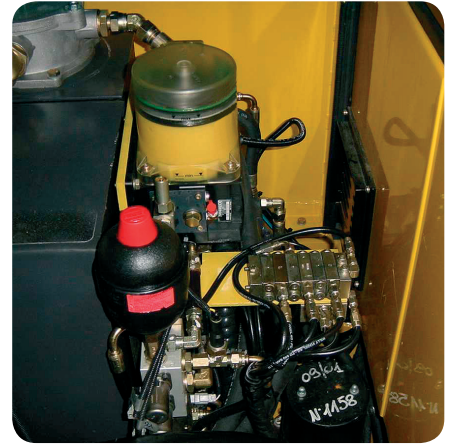
Pump unit with integral control electronics on a KOMATSU PW95.
