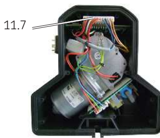
Plug of the control PCB Fig. 21
