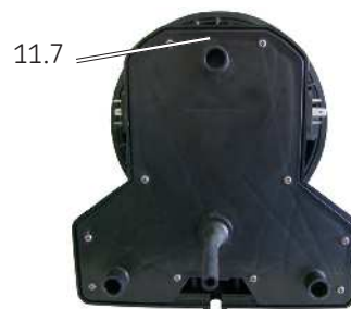
Plug of the control PCB Fig. 25
